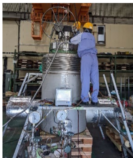
Large Ball Valve for -253°C Cryogenic Liquefied Hydrogen
