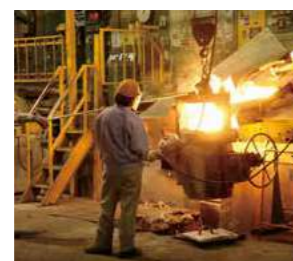
2 Ladling Melted metal is ladled for pouring.
