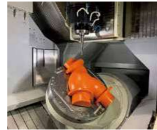
Production of cast molds using the machining center
