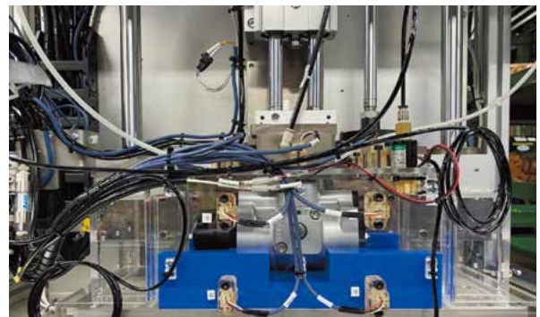
Pressure test of pneumatic actuators with sensors
