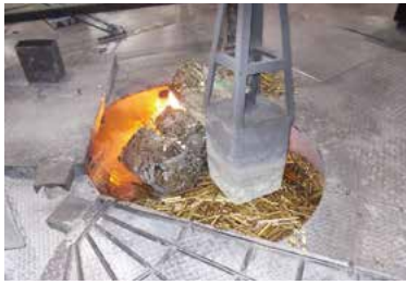
1 Composition and melting of raw materials The raw materials are melted in an induction furnace.
