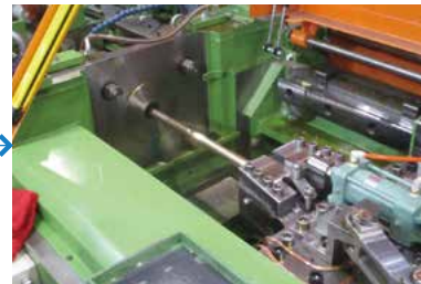
6 Cold drawing The rods and/or coils are passed through the die of a drawing machine to finish them into brass bars with accurate shapes and dimensions.
