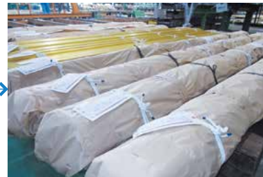
9 Measurement, packing and shipping Completed bars are bundled and packed to the prescribed weight and/or quantity before being delivered to customers.
