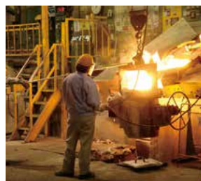
2 Ladling Melted metal is ladled for pouring.
