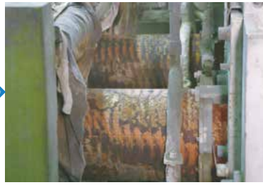
2 Continuous casting The molten alloy is cast into large ingots (called "slabs" or "cakes") using either a water-cooled horizontal continuous casting machine or a vertical semi-continuous casting machine.
