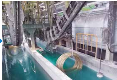
5 Continuous pickling Oxides that have become attached to the surface of the alloy during the extrusion processes are removed by pickling.
