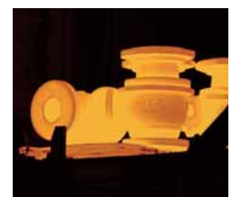
4 Heat treatment (solution heat treatment) Raw materials are quenched after having been heated up to 1,100°C. This process forms a uniform metallic structure and makes mechanical properties such as tensile strength and elongation higher and ensures corrosion resistance.
