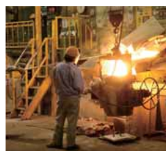
2 Ladling Melted metal is ladled for pouring.
