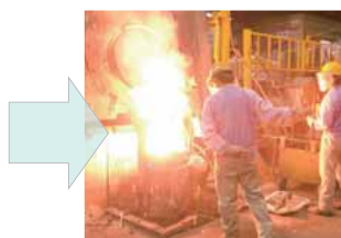
1 Melting Raw materials are melted in high-frequency electric furnaces.
