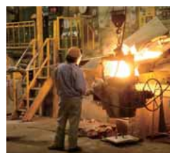
2 Ladling Melted metal is ladled for pouring.
