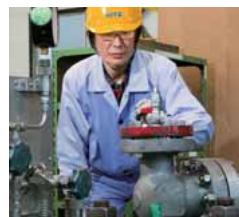
8 Pressure tests Valves are pressurized with air and/or water and operated to verify that they satisfy the quality requirement.
