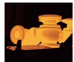
4 Heat treatment (solution heat treatment) Raw materials are quenched after having been heated up to 1,100°C. This process forms a uniform metallic structure and makes mechanical properties such as tensile strength and elongation higher.
