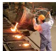
3 Pouring Melted metal is poured into a casting mold. The melted metal flows into the cavity between the upper mold, the lower mold and the core.
