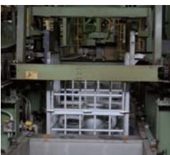
5 Acid pickling Pickling castings in acid solution removes impurities such as oxidized scales on the casting surface caused by heat treatment and shot blasting. At the same time, a protective film is formed on the casting surface for higher corrosion resistance.
