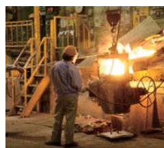
2 Ladling Melted metal is ladled for pouring.
