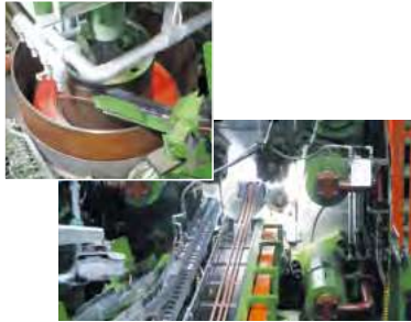
4 Heating and extrusion The billets are heated to the prescribed temperature, and extruded into rods or coils using an extruder.
