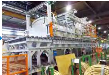
8 Low-temperature annealing The bars are subjected to low-temperature annealing at the prescribed temperature in order to remove residual stress and to adjust their hardness.
