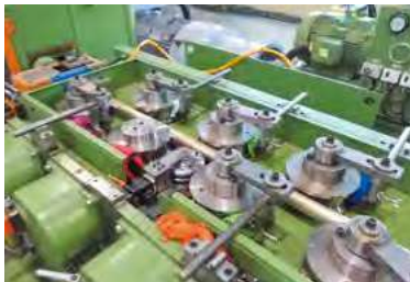
7 Straightening and cutting Bends or curvature in the bars are straightened out using a straightener. The bars are then cut to the prescribed length.
