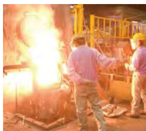
1 Melting Raw materials are melted in high-frequency electric furnaces.
