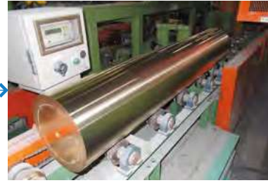
3 Cutting The slabs are cut into billets (intermediate products) of predetermined length ready for extrusion, using a large-scale cutting machine.
