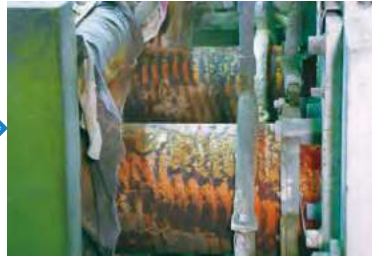
2 Continuous casting The molten alloy is cast into large ingots (called "slabs" or "cakes") using either a water-cooled horizontal continuous casting machine or a vertical semi-continuous casting machine.
