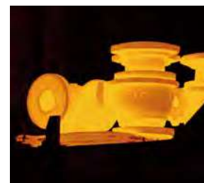
4 Heat treatment (solution heat treatment) Raw materials are quenched after having been heated up to 1,100°C. This process forms a uniform metallic structure and makes mechanical properties such as tensile strength and elongation higher and ensures corrosion resistance.
